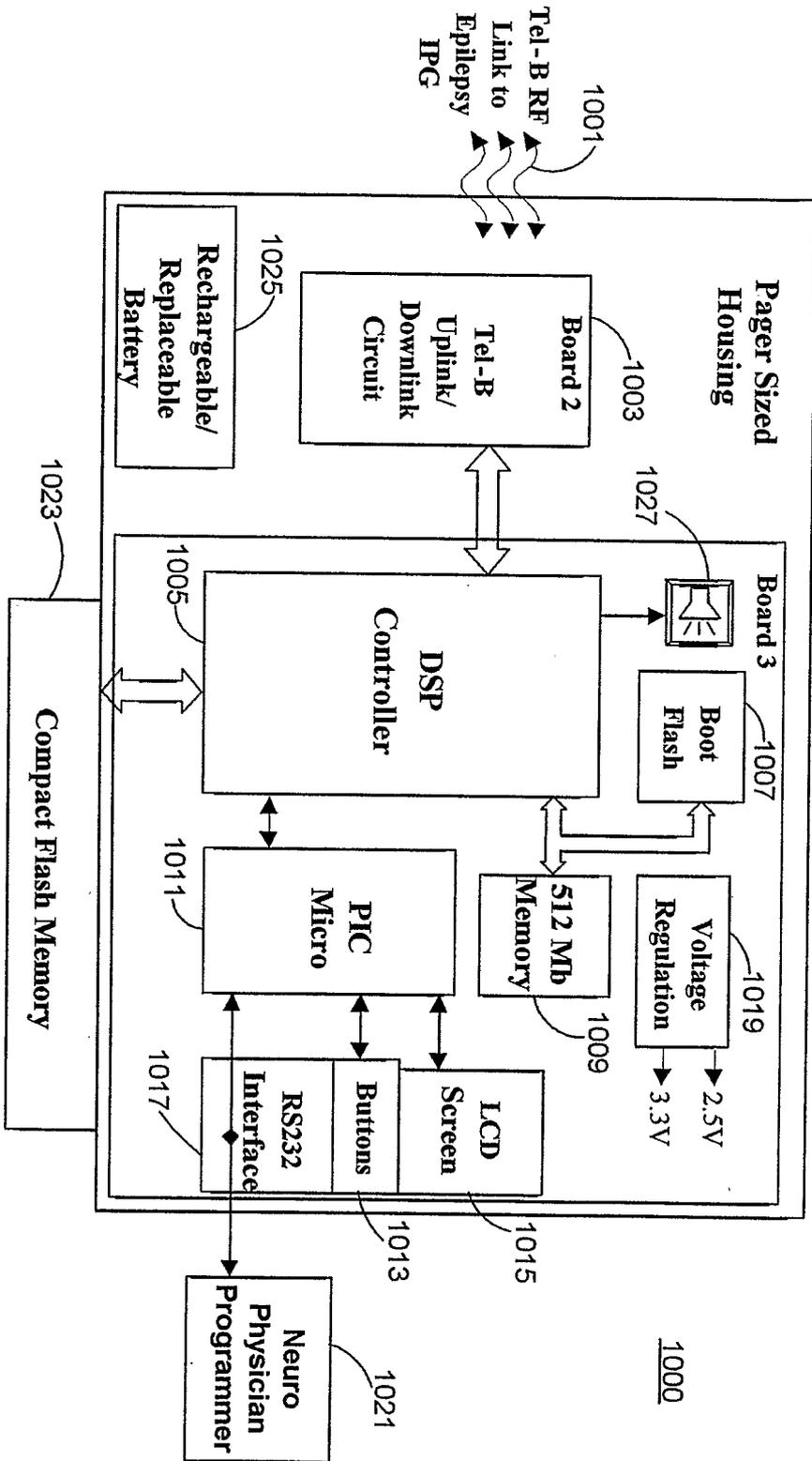
FIG. 10 (Epilepsy external device diagram)
