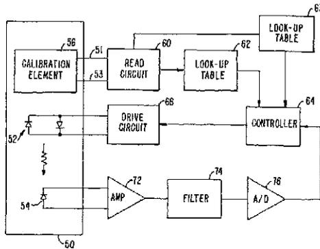
(57) Abstract: The present invention provides a memory chip for use in an oximeter sensor, or an associated adapter or connector circuit. The memory chip allows the storing of patient related data, such as patient trending data or a patient ID, to provide enhanced capabilities for the oximeter sensor. In addition to providing unique data to store in such a memory, the present invention include unique uses of the data stored in such a memory.
