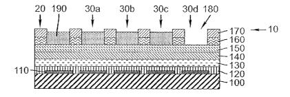
(57) Abstract: A method of making an OLED display having a plurality of OLED devices includes providing a plurality of OLED devices on a substrate, such OLED devices sharing a common light-transmissive electrode; forming a patterned conductive layer structure over the common light-transmissive electrode to define wells in alignment with emissive areas of one or more OLED devices; and providing optical material into one or more wells.
