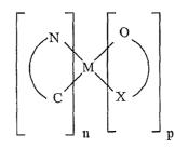
wherein M is a heavy transition metal; C--N is a cyclometallated ligand; O--X is a coordination ligand wherein X is selected from the group consisting of oxygen, nitrogen, and sulfur; and wherein n equals 1 or 2, and p equals 0 or 1.
