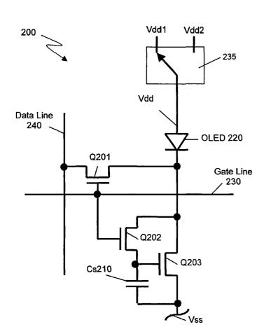
(57) Abstract: There is provided a method for driving an organic light emitting diode (OLED) pixel circuit. The method includes applying a first signal (Vdd1) to a terminal of the OLED (220) when setting a state of the pixel circuit (200), and applying a second signal (Vdd2) to the terminal when viewing the state. There is also provided a driver (235) for an OLED pixel circuit, where the driver employs this method.
