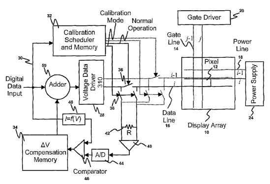
(57) Abstract: A method and system for programming, calibrating and driving a light emitting device display is provided. The system may include extracting a time dependent parameter of a pixel for calibration.
