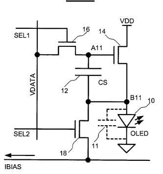
(57) Abstract: Active matrix light emitting device display and its driving technique is provided. The pixel includes a light emitting device and a plurality of transistors. A capacitor may be used to store a voltage applied to a driving transistor so that a current through the light emitting device is independent of any shifts of the transistor and light emitting device characteristics. A bias data and a programming data are provided to the pixel circuit in accordance with a driving scheme.
