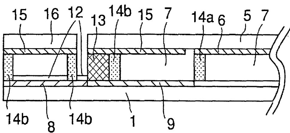
**LIQUID-CRYSTAL DISPLAY DEVICE HAVING A SHIELD SHIELDING AN ELECTROMAGNETIC WAVE RADIATED FROM ONE OF A DRIVER AND AN ELECTRODE LEAD-OUT LINE**
