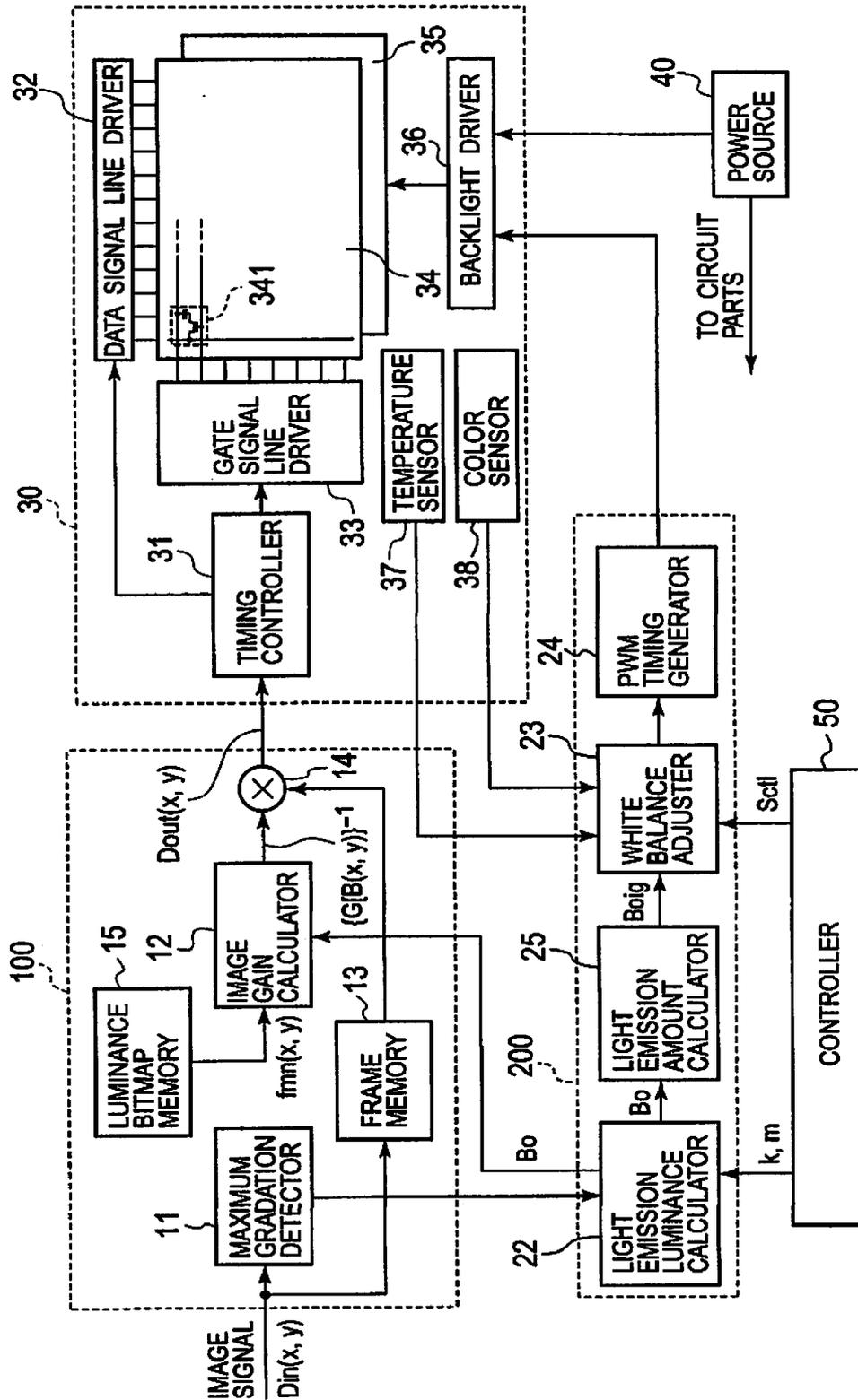
**FIG. 35A**  $d_{out}(x, y) = \frac{G^{-1} [ D_{in}(x, y) ]}{B(x, y)}$  ... (32)
