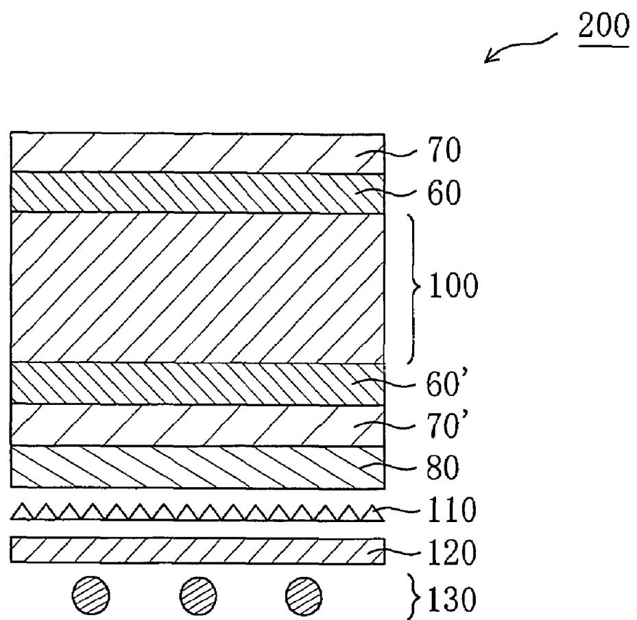
**LIQUID CRYSTAL PANEL AND DISPLAY APPARATUS HAVING A NEGATIVE BIAXIAL ELEMENT OF 110 TO 250 NM THICKNESS DIRECTION RETARDATION VALUE AND AN NZ COEFFICIENT OF 1.4 OR MORE**
