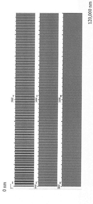
Interference color chart calculated using emission spectrum of cold-cathode tubes (retardation = 0 to 120,000 nm)
