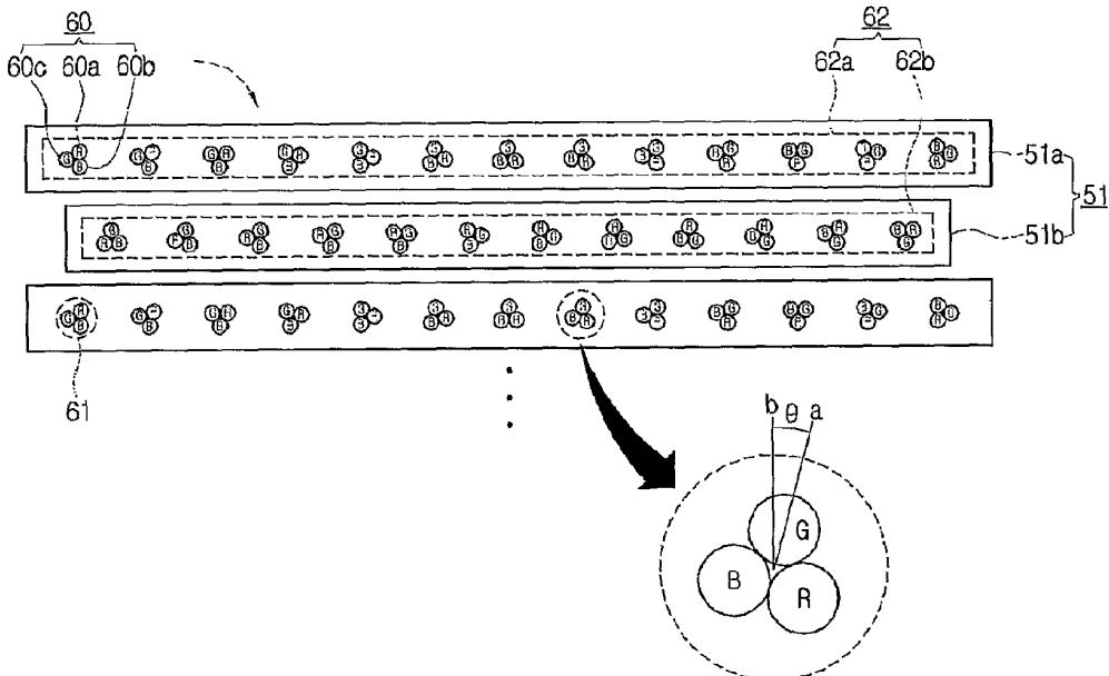
(57) Abstract: A backlight unit is provided. The backlight unit includes a point light source circuit board and a point light source group row comprised of a plurality of point light source groups arranged in the point light source circuit board in a line. In addition, at least a part of the point light source groups have a different rotating angle with respect to each other.
