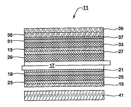
substrate (35) is bonded to the front of the front polarizer by the above-mentioned sensitive adhesive. An anti-reflection coating (39) is applied to the front of the third glass substrate. A backlight (41) is positioned behind the second glass substrate.
